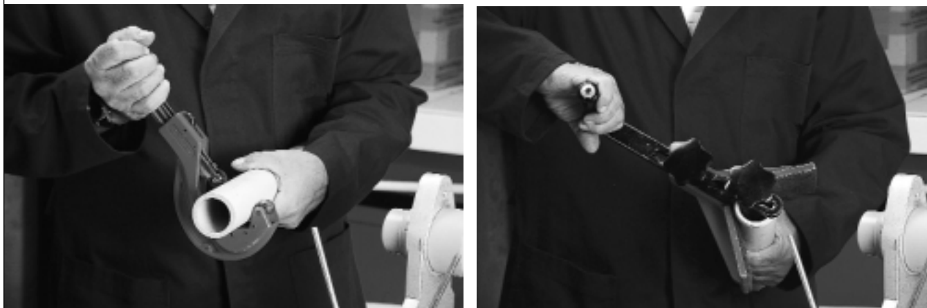
Polypropylene Fittings for Socket Welding. Chamfer dimensions.
